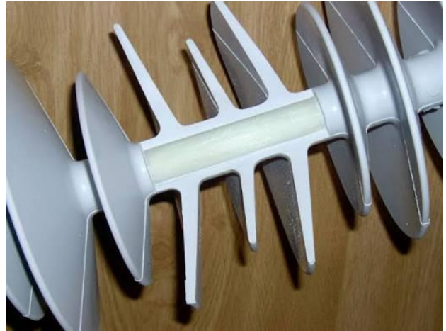
Figure 2. HTV composite silicone insulator
