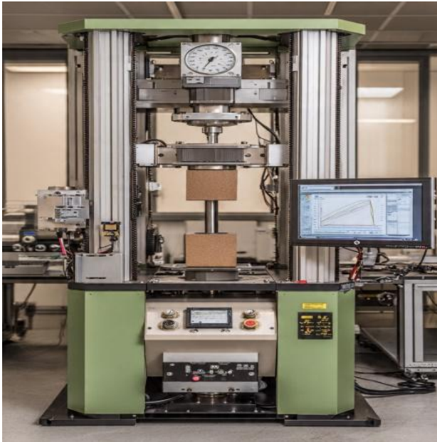
Figure 4. Experimental setup for flexural testing
