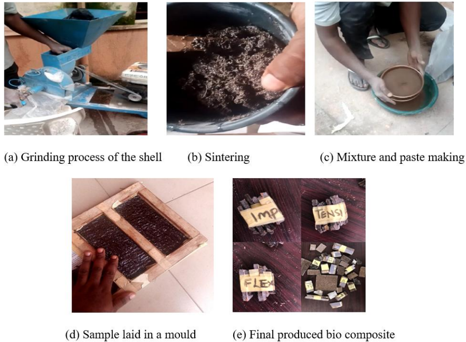
Figure 3. Process development of the biocomposite
