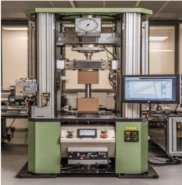
Figure 4. Experimental setup for flexural testing
