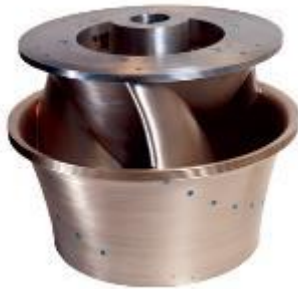
Figure 10. Physical model of an Alden turbine runner [51]
