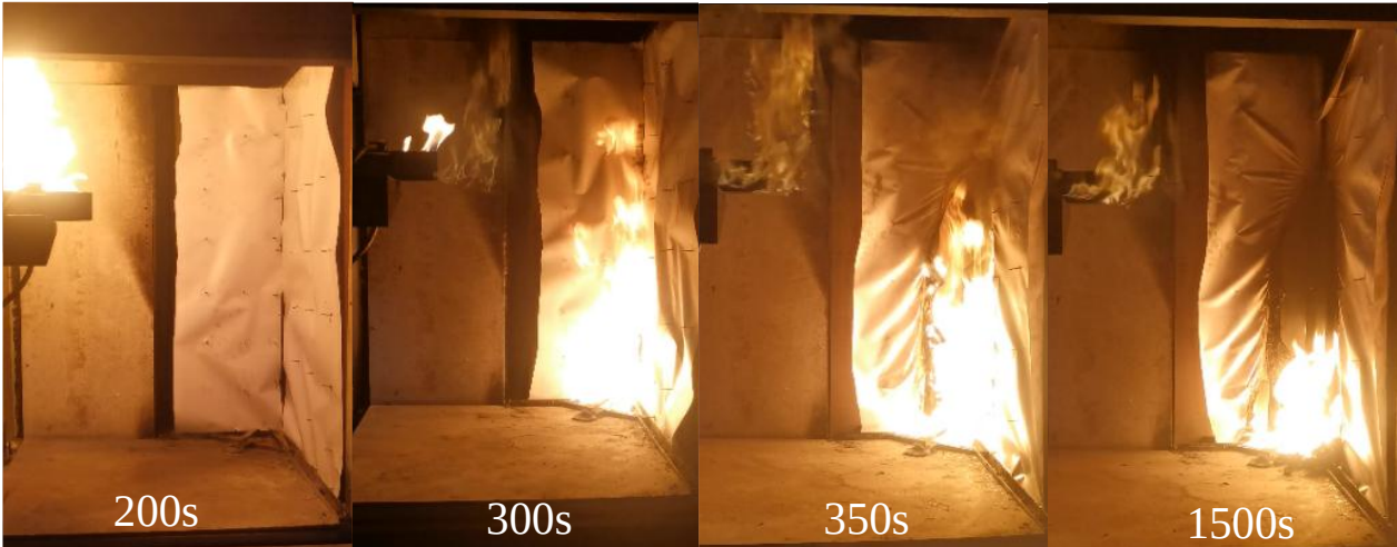
Figure 10. Combustion process diagram of PVC4
