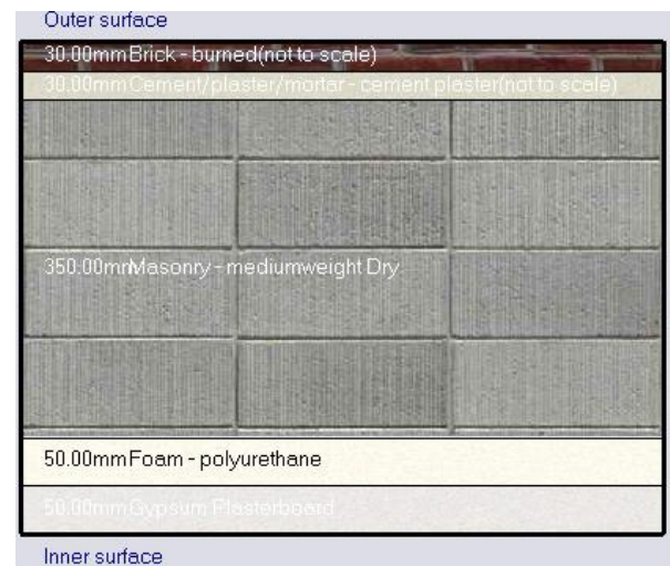
Figure 10. External walls structure
