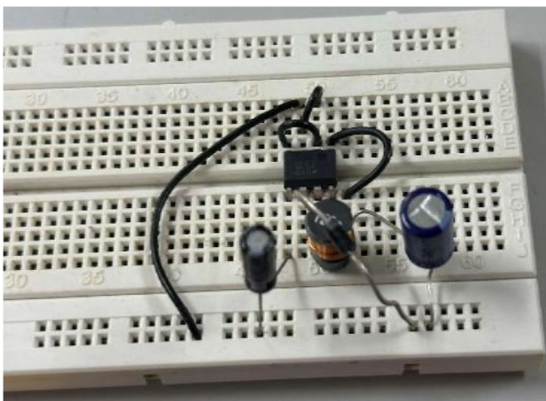
Figure 4. Buck converter breadboard prototyping with the LM2574 500mA IC for troubleshooting
