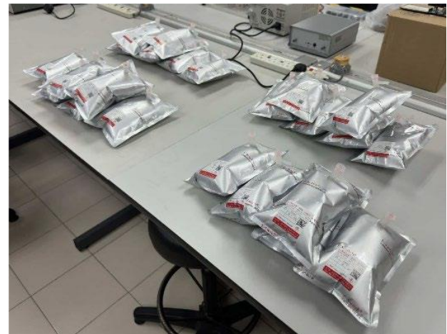
Figure 8. Sample collection using Tedlar bags with a total of 75 air samples
