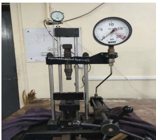
Figure 8. Universal testing machine
