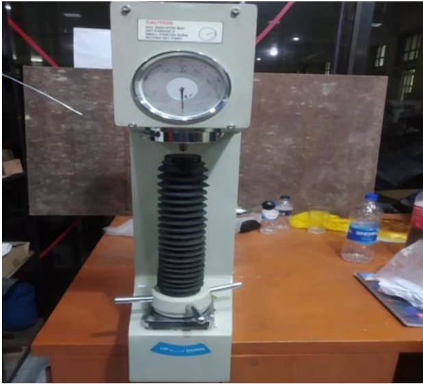
Figure 11. Hardness testing machine
