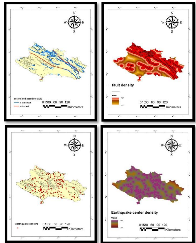
Figure 2. Map of Lorestan active and inactive fault layers, standardization of the density layer of Lorestan faults, Lorestan earthquake centers, and standardization of the density layer of earthquake centers
