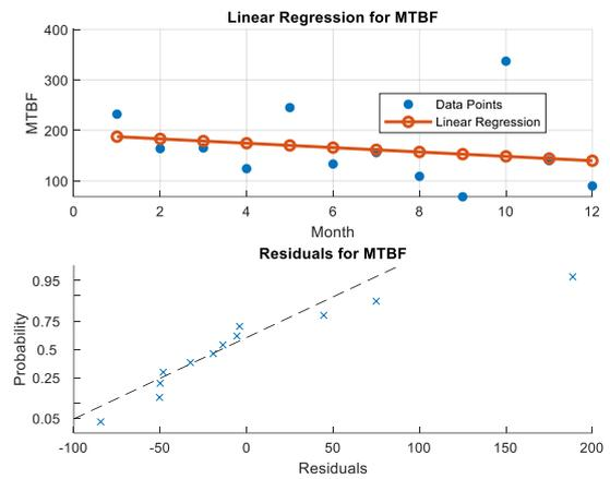
Figure 5. Linear regression plot of mean time before failure
