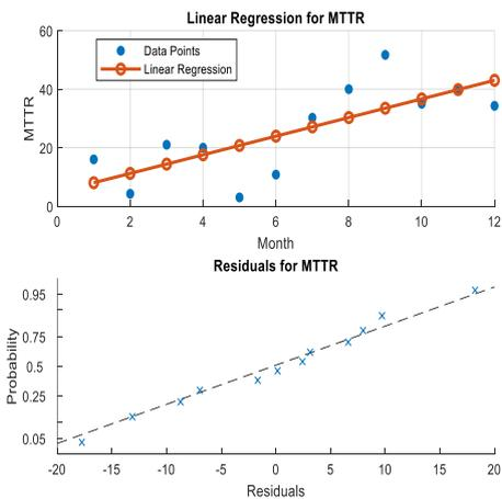
Figure 2. Linear regression plot of mean time to repair
