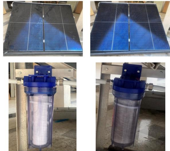
Figure 14. Influence of the cleaning system on both PV panels and the water filter: (a) Before water runoff; (b) After water runoff
