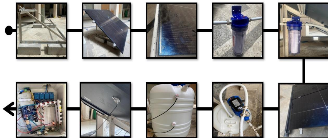
Figure 8. Hardware and software description of the cooling and cleaning system for two PV panels
