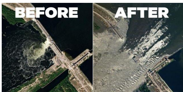
Figure 1. Aerial photographs of the Nova Kakhovka dam, Ukraine, before and after failure (Google Earth accessed on 15 December 2022)
