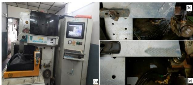
Figure 6. (a) Electronica sprint cut wire EDM setup, (b) Fixing of Nimonic alloy 75 sheets on Wire cut EDM table, (c) Machined Nimonic alloy 75 sheets
