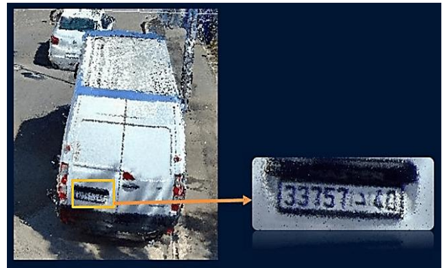
Figures 13. The high-definition capture capability of the LiCam, providing clear visual identification of license plates from Car 2
