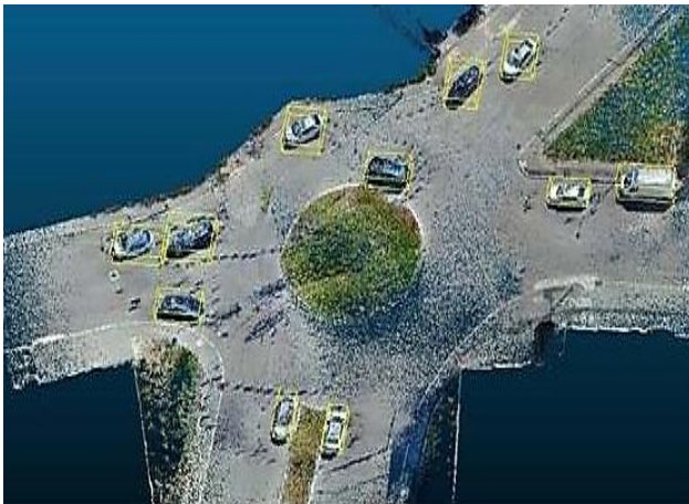
Figure 16. The local dataset acquired over a 2-hour duration with a relative measurement accuracy of \pm 2 cm
