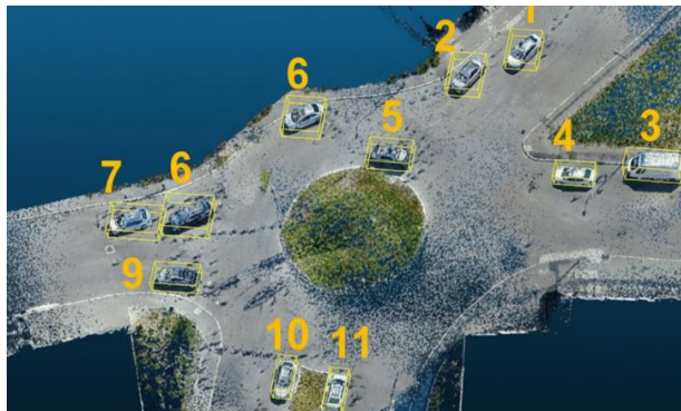
Figure 8. Result of automatic counting with DBSCAN
