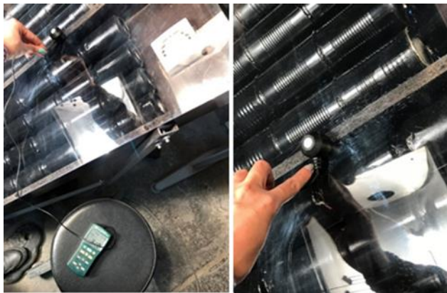
Figure 3. Radiation intensity measurement by model radiometer TES
