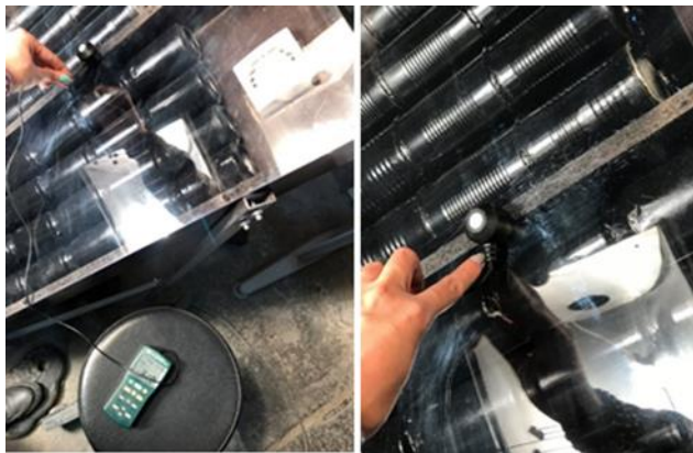
Figure 3. Radiation intensity measurement by model radiometer TES
