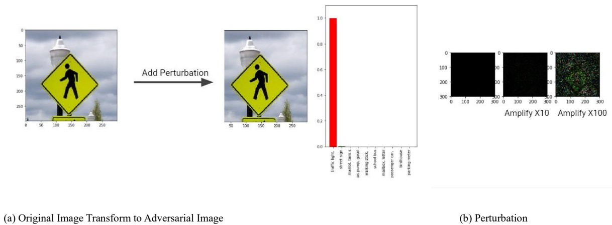
Figure 10. Incorrect classification of a street sign using an adversarial image
